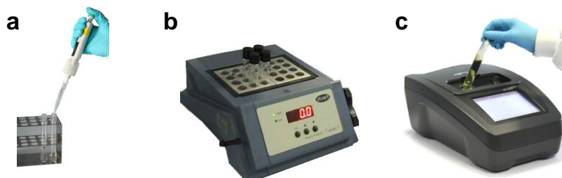
Figure 2: OMMICA™ method for water samples, a) add reagents and sample to tube, b) heat and c) analyse in spectrophotometer.
